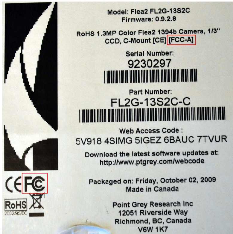
Figure 2: Camera box label with FCC logo and FCC part-number declaration outlined in red
